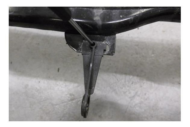
25. Fit the temperature sensor and its bracket to the Forge bracket from the FMINT33 kit. Using a 6mm Allen key and the supplied M8 fastener attach the temperature sensor to the intercooler and plug the loom as shown in the pictures below.
