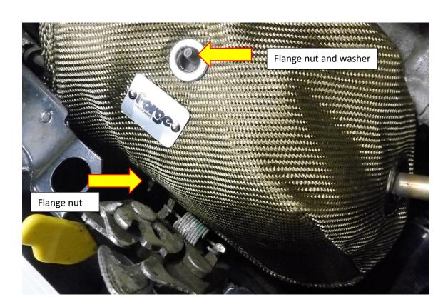
**11**. Using a 5mm Allen key secure the top half of the turbo blanket using the 3x supplied M6 Allen cap fasteners and washers. If you are still running your dump valve as a recirc remember to re fit the pipe bracket here.
