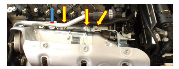
6. Using a T30 Torx driver remove 3x M6 Torx fasteners. Using a 10mm spanner remove the M6 nut at the lower front section of the OE heatshield. The front section of the OE heat shield can now be removed.
