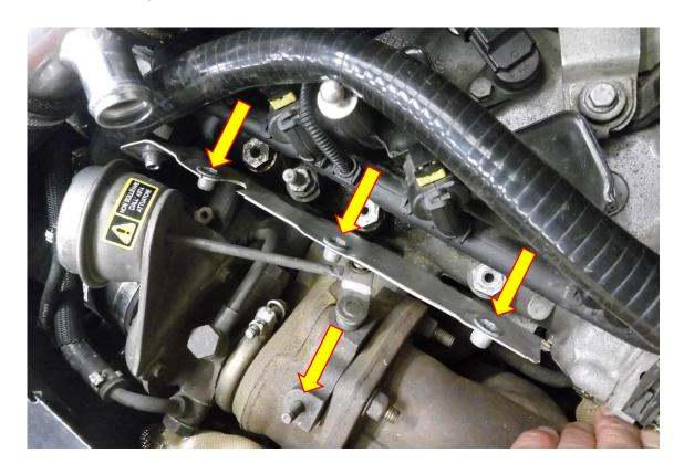
8. Using some plyers bend the corner of the OE heat shield bracket this is to avoid the blanket being damaged.
