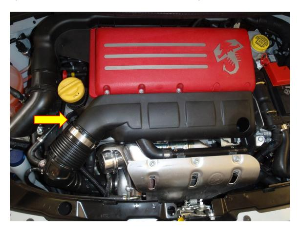
3. Release the DV pipe from its mounting points and using a flat blade screw driver release the hose clamp attaching the rubber hose to the DV pipe.
