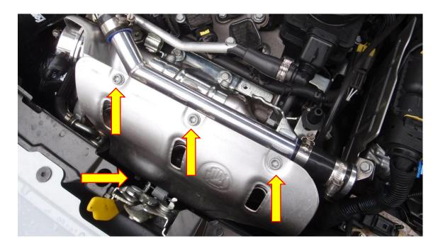
7. Using a T30 Torx driver remove the 4x M6 Torx fasteners to allow removal of the back half of the OE turbo heat shield.
