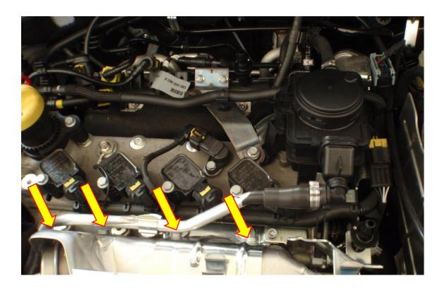
With both parts of the heatshield removed this is how it should look. The arrows shows where you are to secure FMTUBL16 in place.
