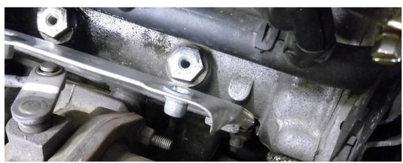
9. Depress the yellow locking clip and un-plug the lambda probe loom. Feed the lambda plug through the large hole on the FMTUBL16.
