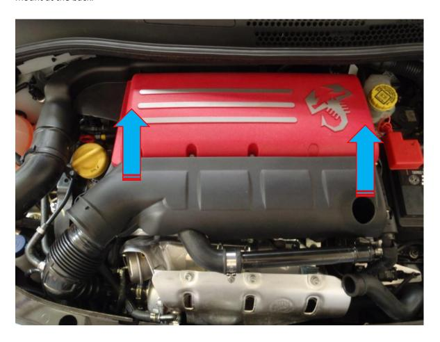
5. Using a 10mm spanner remove the 2X M6 fasteners and using a T30 Torx drive remove the 1x N6 Torx fastener. Un-clip the oil breather pipe.
