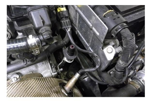
10. Fit the turbo blanket in place, start at the bottom and secure using a 10mm spanner and one of the supplied flange nuts. Use a flange nut and washer for the upper mounting point.
