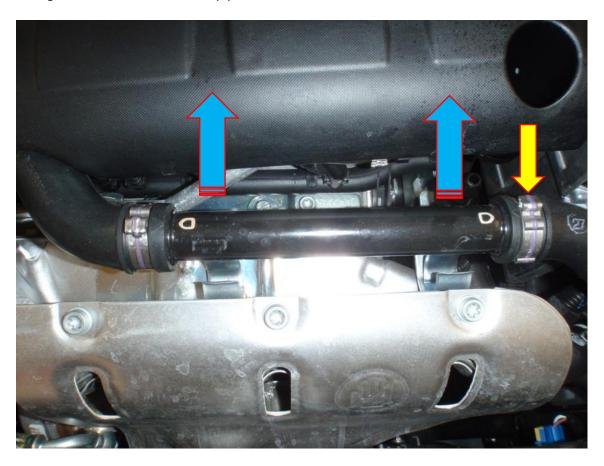
4. Pull the filter box upwards with an even pressure at the front until it has come away from its rubber mounts. Then pull upwards with an even pressure the back of the filter where indicated to release from the rubber mount at the back.
