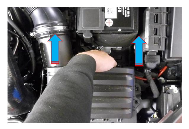
1. If your vehicle is equipped with this type of battery clamp follow these next four steps, if it's not go straight to step four. Using a 10mm socket and ratchet disconnect both battery terminals, start with the negative battery terminal and use the negative terminal cover to stop it touching the terminal when removing the positive side.
