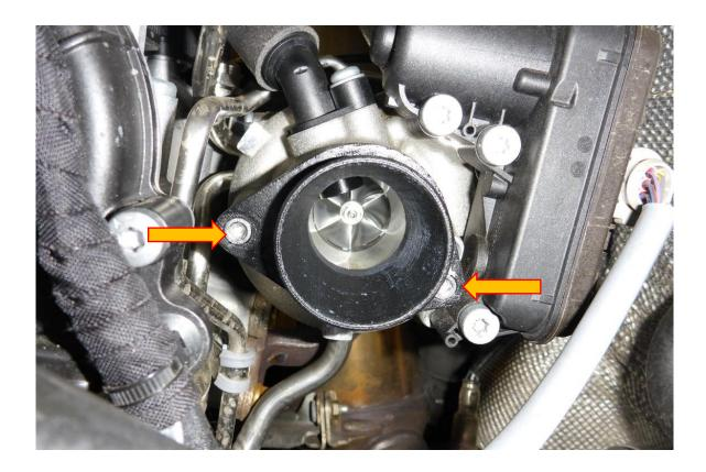
9. Fit the Forge silicone intake hose to the turbo adaptor, using a 7mm socket and rachet or a flat bladed screwdriver fit the 50-70 hose clamp to secure it in place.
