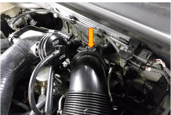
2. Pull the air box upwards sharply so it releases from its rubber mounting points and remove it and the attached intake pipe completely from the vehicle.
