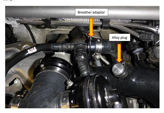
If your vehicle is not equipped with the extra breather hose, use the remaining alloy blanking plug to block off the spout and secure with the 16-27 hose clamp.
