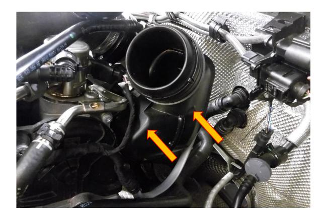
6. With the use of long nose plyers push in the two tabs while pulling the adaptor to free it. Remove the breather hose adaptor from the OE turbo elbow
