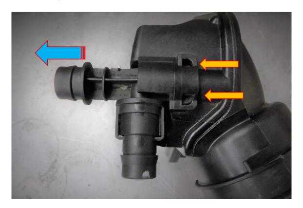
7. With the breather adaptor now removed, take the Forge Motorsport billet breather adaptor, and push it onto the end of breather adaptor with the green O ring. There is location marker on the billet adaptor which must be lined up with the plastic moulded line as shown in the picture below. Use the U clip supplied to secure the billet adaptor in place.
