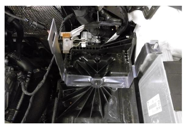
**4.** Release the two Norma fittings attaching the breather hoses to the turbo elbow. If your vehicle is not equipped with this system ignore the rest of the breather system steps.
