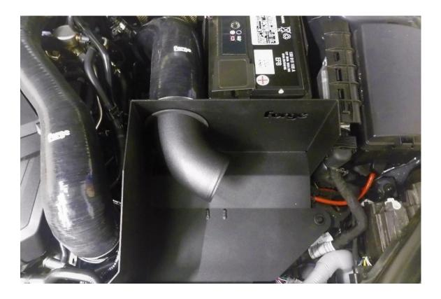
13. Fit the Forge filter onto the end of the alloy pipe and secure it into place with the remaining 70-90mm hose clamp. Angle the filter so that it has between 10mm-15Mmm clearance from the bottom the filter tray, then tighten the other hose clamp fitted in step 11. Use a 7mm socket and rachet or flat blade screwdriver to tighten the hose clamps.
