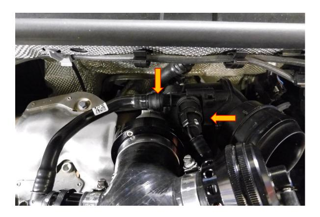
5. Using a T30 rachet and suitable extension remove the two T30 fasteners attaching the OE turbo elbow to the turbo charger
