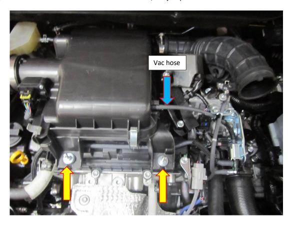
4. The MAF sensor will now need to be removed, first unplug the sensor then remove the two Philips screws attaching it to the air box using a Philips screwdriver. Now carefully remove the sensor from the air box. Un clip the MAF wiring harness.
