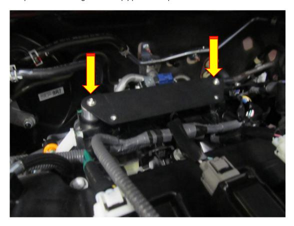
9. Take the hard pipe from the kit and mount the original MAF sensor into the MAF boss on the hard pipe, there are two m4 fasteners with kit with the use of a 4mm Allen key tighten the sensor to the MAF boss.
