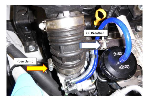
6. At this stage you can now remove the whole air box and pipe work as one, lift the back of the air box to release it from its rubber mounting points. Make sure all the vac hoses a un attached from the intake pipe and you will be able to remove the air box. To do this pull out the air box while twisting it 90 degrees to the left as shown in the picture.
