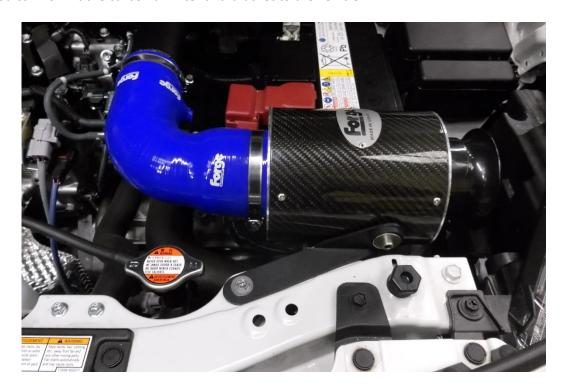
**19.** Finally go back to the mounting bracket and tighten the M6 fasteners and all the hose clamps for the silicone hoses.
