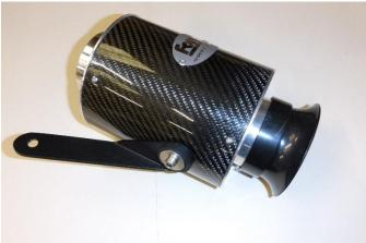
18. You can now fit the carbon air filter and bracket to the vehicle
