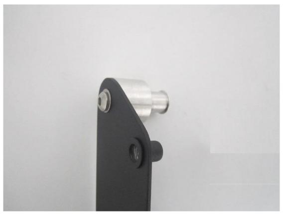
8. Once you have made up the mounting bracket, install it into the rubber lugs that held the back end of the airbox in place. The mounting bracket simply pushes into place.
