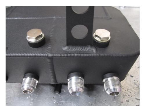
5. Fit the FMCT5 into the same location as the OE expansion tank, fit the lower coolant pipe using the original hose clamp. Secure the tank into place with the fasteners used to hold the OE tank as shown in the picture below
