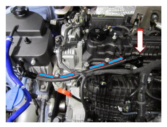
9. Attach the AN-6 fitting of the smaller hose to the catch tank and run the hose to the rocker cover as shown in the picture below. Use a 17mm spanner to tighten the AN-8 fitting and a 7mm socket to tighten the hose clamp on the breather end of the hose.
