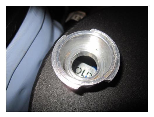
13. Take your original coolant cap and screw onto the Forge expansion tank. Once fully tightened place the Forge alloy cap over the OE cap line it up and fix into position with the grub screw.
