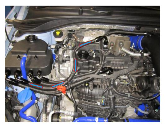
**12.** Re fill your coolant into the expansion tank, there is a maximum level indicator, the coolant should be just below this indicator. You may need to top this up after a few miles due to the system still bleeding any trapped air.
