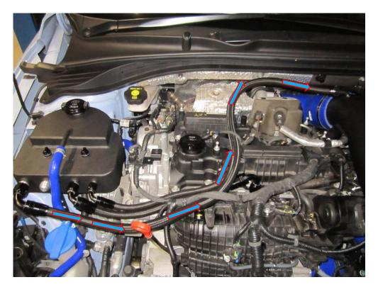
**11**. The last hose to be installed is another AN-10, run the hose as shown in the picture. The breather end is another push fit.
