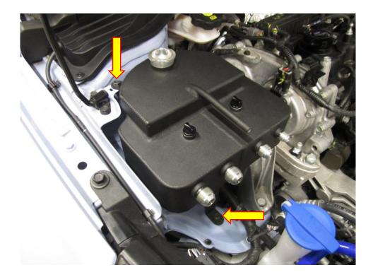
6. From the FMCT5 kit, take the two rubber grommets and two alloy fittings. Make sure that the plane rubber gromet is inserted into the short fitting and the ribbed rubber gromet is fitted to the taller alloy fitting. Now fit each fitting to the appropriate 120 degrees dash fitting from two of the braided hoses from the kit. They can only fit one hose as they are different thread sizes. Use a 26mm spanner and an adjustable spanner to tighten.
