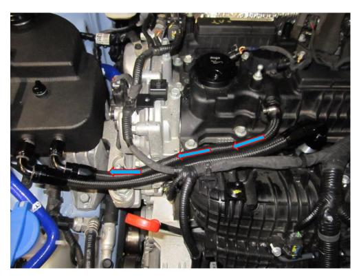
10. Take the longest hose from the kit and run the hose as shown in the picture below. Unclip the wiring loom to the injector behind the oil cap, this will allow you to run the hose underneath it, then re connect the loom. Use a 25mm spanner to tighten the AN-10 fitting and a 7mm socket for the hose clamp at the other end of the hose.
