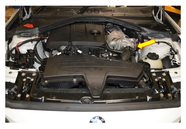
2. Using a T30 Torx drive remove the three fasteners that hold the OEM valve in position and disconnect the wiring loom.
