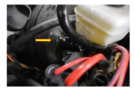
7. Connect the vacuum hose provided to the vacuum take off adaptor and run the length of hose to the Forge Motorsport valve as pictured below ensuring it does not foul the wiper mechanism.
