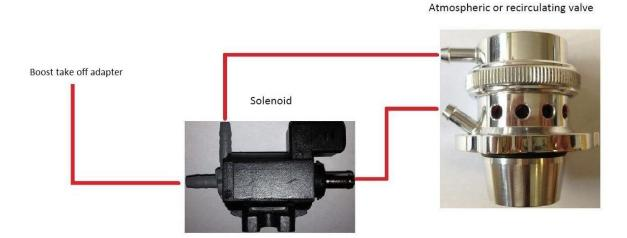
9. Connect the OEM wiring loom to the solenoid provided as pictured below and fix the solenoid in position using a cable tie provided.
