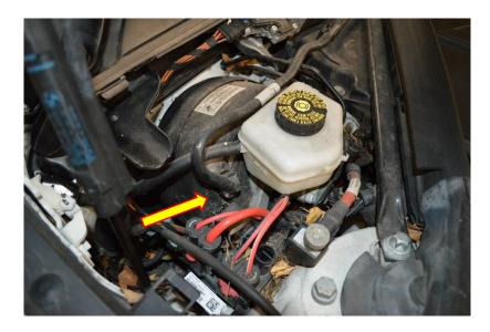
6. Push the Forge Motorsport vacuum adaptor into position then reinstall the brake servo pipe into the adaptor and rubber gromet.
