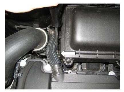
Remove the MAP sensor from the top of the inlet manifold as shown, then push it firmly into the supplied Forge MAP sensor boss. A little silicon spray will make it easier. You can then attach the hose from your boost gauge to the takeoff on the block, then reattach the whole assembly back to the inlet manifold with the screw provided, and refit the airbox and hoses removed
