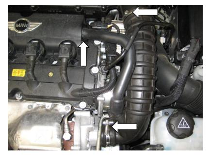
Lift the bonnet and begin by undoing the two jubilee clips holding the hose between the airbox and turbo inlet.
