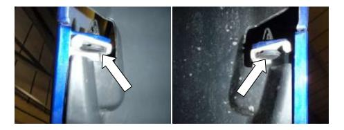
11. Pull the arch liner outside of the front bumper, to allow the bumper to pull forward without catching.
