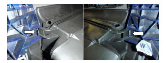
17. To remove the stock intercooler undo the 2x 8mm bolts located underneath the intercooler.
