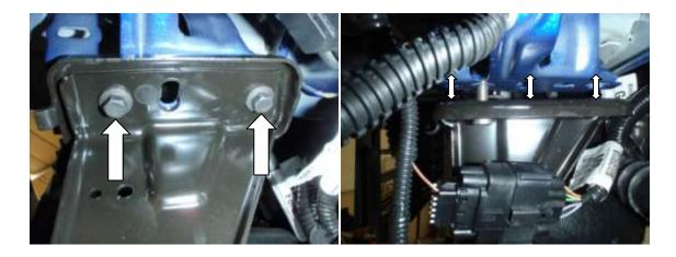
21. This allows the radiator to move downwards, disconnect the large connector (passenger side) for the active ducting. Lift the plastic ducting upwards to unclip it from the radiator.
