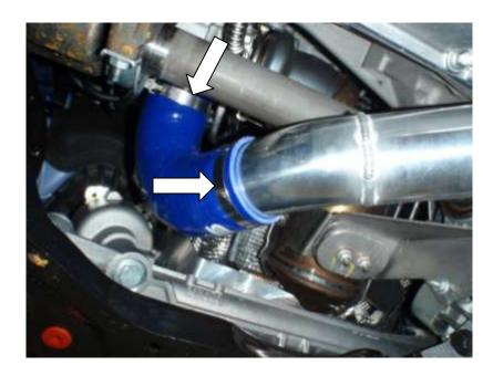
35. Use the remaining 90Deg silicone hose to connect the hard pipe to the intercooler outlet. Secure with suitable hose clamps.
