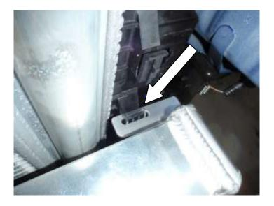
26. Using an M6X16mm Hex head bolt, 3x M6 washers and 2x M6 Nyloc nuts bolt the bottom mounts to original intercooler mounts.
