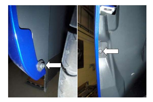
9. Undo the 2x T30 Torxs located underneath in front of both wheels.
