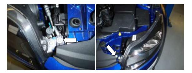
5. To release the headlights undo 2x T30 Torxs, pull the headlight forward unclip the large connector at the rear of the headlight. You may need to pull the bumper forward to allow the headlight to clear the edge of the bumper. Store the headlights in a safe place to prevent damage, while working on the rest of the vehicle.
