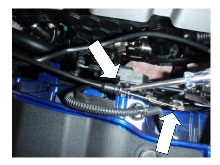
7. Using a flat blade screwdriver or similar tool remove the four plastic clips along the top edge of the bumper.
