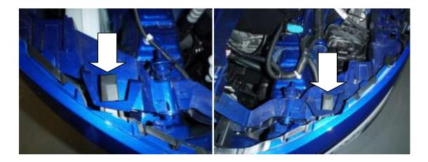
15. To remove the lower plastic air duct undo the 2x T30 Torxs and unclip from underneath.
