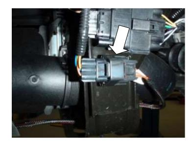
22. On the standard intercooler remove the MAP sensor using a T20 Torxs.
