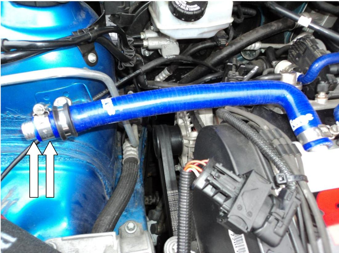
9. Now fit the oil breather filter onto the 19mm hose joiner along with a hose clamp and tighten.
