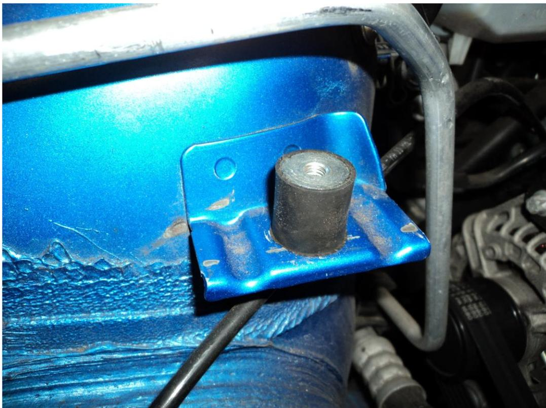
8. Fit the new Forge breather hose to the outlet on the cam cover and tighten with a hose clamp. At the opposite end fit the "P" clip to the pipe along with the bolt supplied and bolt to the cotton reel. You will also need to place the 19mm hose joiner into the end of the pipe and tighten with a hose clamp.
