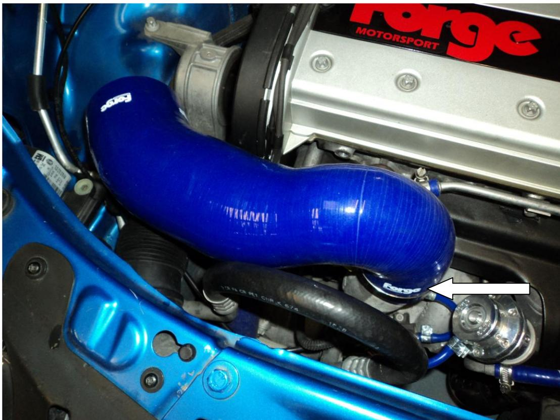
11. Next you will need to fit the air flow sensor into the other end of the intake pipe. Please make sure the arrow on housing is pointing the same way as in the picture.
