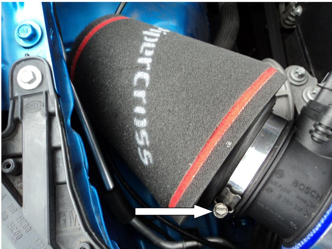
13. Place the air flow sensor plug along the top of the cam cover as seen in the picture below and using the cable tie, tie up wire to the others.
